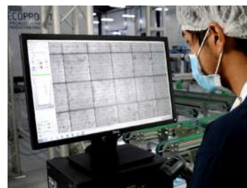
NEURAL NETWORK SOFTWARE FOR AUTOMATIC DETECTION OF DEFECTS
